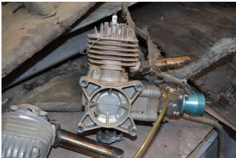
Figure XIV 3W-110i B2 engine inspected in Ma'rib
