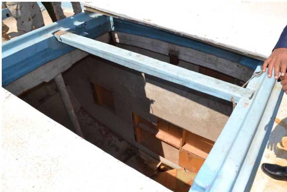
Figure VIII Hidden cargo compartments on the Bari-2 used to smuggle weapons
